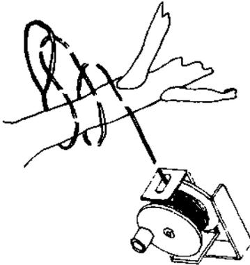
**Primary Tie-off** - with an unobstructed ascent to the surface - pass the reel through the loop and then make an additional wrap - pull in all directions to make sure the anchor is secure
