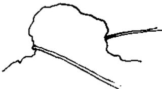
**Line Placement** - the line is routed around a projection to keep it in place and prevent it from going into a line trap
